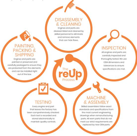
Our advanced remanufacturing process brings worn engines and parts back to life, resulting in significant benefit for you and the environment.
