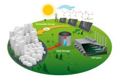
As long as sufficient electricity from solar and wind power is available or energy prices are low, the CHP system reduces load, and the pre-stored heat supplies the city with district heating.
